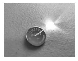
**1.1** Test your LEDs one at a time. Remember to place the positive (+) leg of each LED on the positive side of your battery and the negative (-) leg on the negative side.
