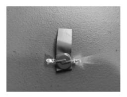
**2.2** Cut a 3-inch piece of electrical tape and wrap it once around the battery and LED legs. Make sure the tape is securely attached to the battery and only wrap it around the battery once. Leave the extra tape loose.
